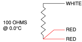
SINGLE 3 WIRE CONSTRUCTION
